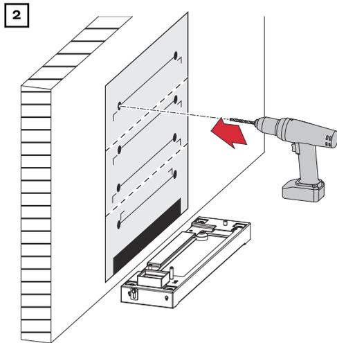
Drill holes at the required fastening points.
