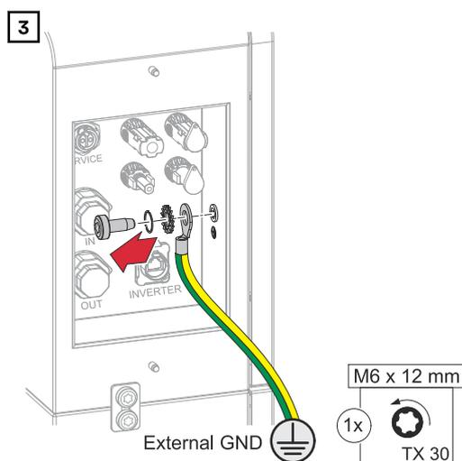
Loosen the ground conductor using a screwdriver (TX30).
