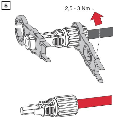
Tighten the cable gland using the supplied Amphenol plug tool to a torque of 2.5 Nm - 3 Nm.
