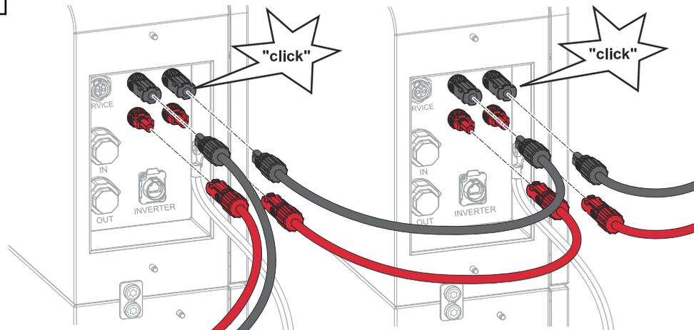
Insert the Amphenol plugs (+/-) into the respective slot until they engage.
