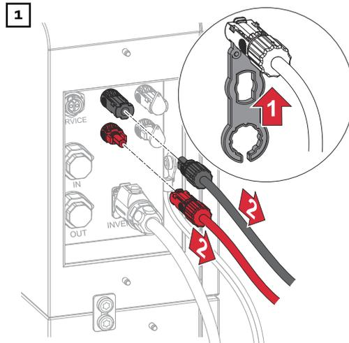
Loosen the Amphenol plugs (+/-) using the Amphenol plug tool.
