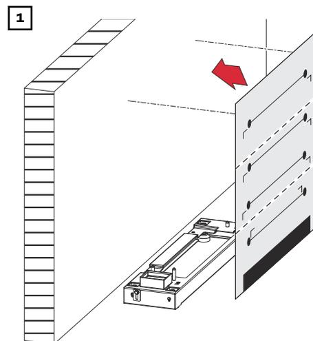
Align the drilling template horizontally on the wall and stick it on.
