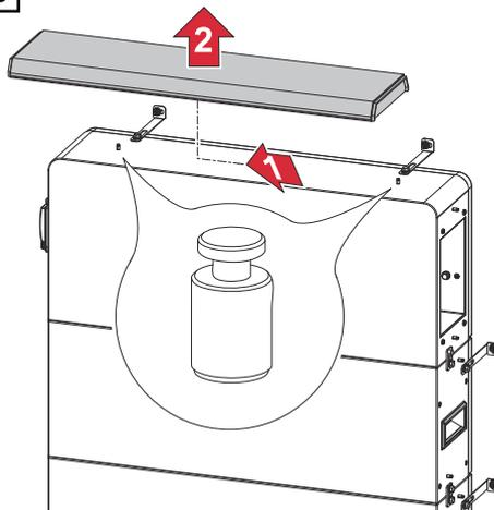
Slide the top cover on the Reserva BMS to the left and lift off.
