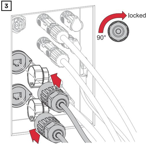
Connect the data cable to the "IN" (data input) or "OUT" (data output) data communication connection and rotate 90° to the right.
