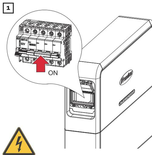
Turn the DC disconnect of the battery to the "On" switch setting.
