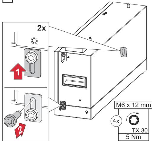
Fasten the 2 connecting tabs using the screws supplied (TX30) and to a torque of 5 Nm.
