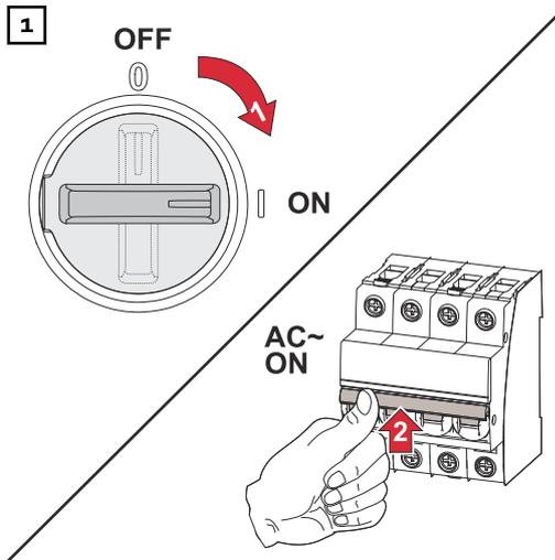
Turn the DC disconnecter of the inverter to the "On" switch setting. Turn on the automatic circuit breaker.
