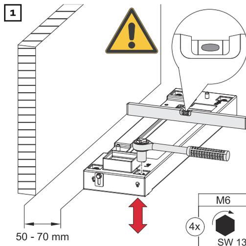
Position the base plate parallel to the wall at a distance of 50 - 70 mm and align it horizontally by turning the adjusting feet with a socket wrench (width across flats 13).
