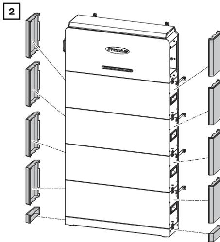
Push in the side covers from above, starting with the base plate, until the covers engage.
