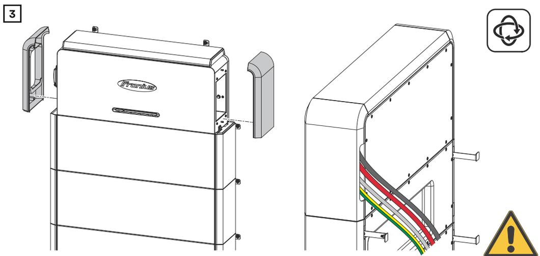
Push in the side covers of the Reserva BMS from above until the covers engage. Feed the cables through the side cutout in the cover.
