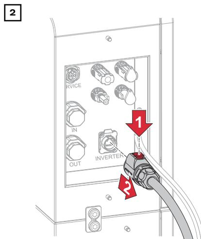
Press the locking mechanism on the plug of the "INVERTER" data cable and remove the plug.
