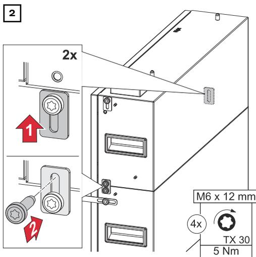
Fasten the 2 connecting tabs using the screws supplied (TX30) and to a torque of 5 Nm.
