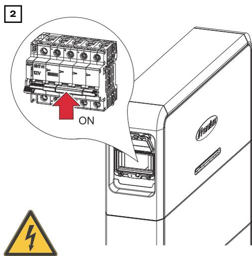
Turn the DC disconnecter of the battery to the "On" switch setting.
