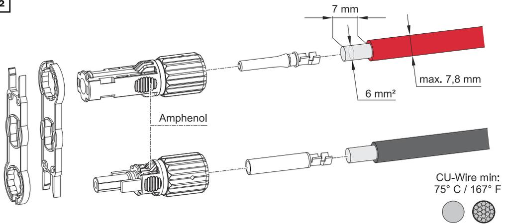
Select the cable cross-section in accordance with the instructions in [Permitted cables for the electrical connection](#) on page 32. Strip the insulation of the single conductors by 7 mm (0.27 inch).
