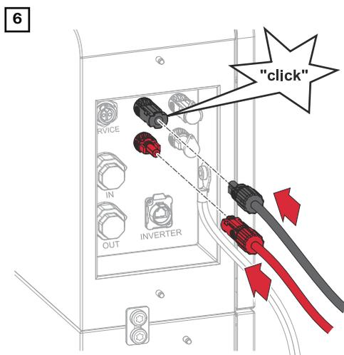
Insert the Amphenol plugs (+/-) into the respective slot until they engage.
