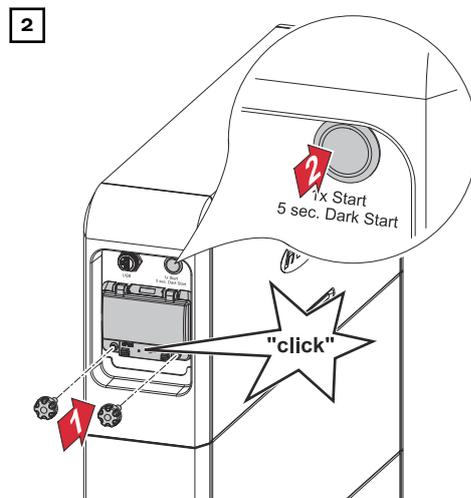
Close the cover of the DC disconnect until there is an audible click and secure it against unauthorized opening with the screws. Press and hold the start button for 5 seconds to start the battery.
