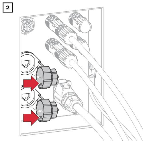
Remove the closure caps of the data communication connections "IN" (data input) or "OUT" (data output) by rotating them 90° to the left.
