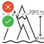
The battery must not be installed or operated at more than 2,000 m above sea level.
