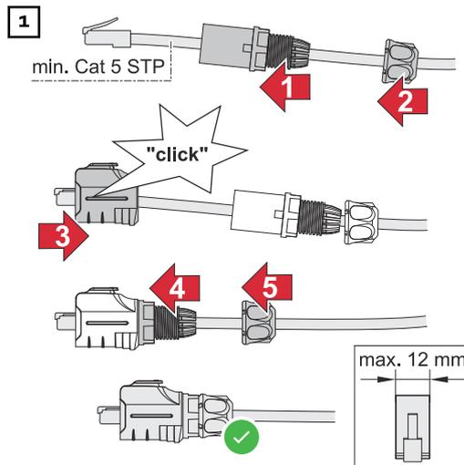
First, guide the data cables through the union nut and then through the cable gland. Insert the plug insert until there is an audible click. Fasten the union nut to the cable gland.
