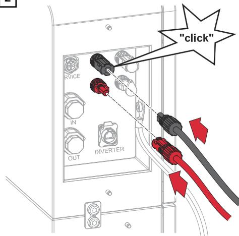
Insert the Amphenol plugs (+/-) into the respective slot until they engage.
