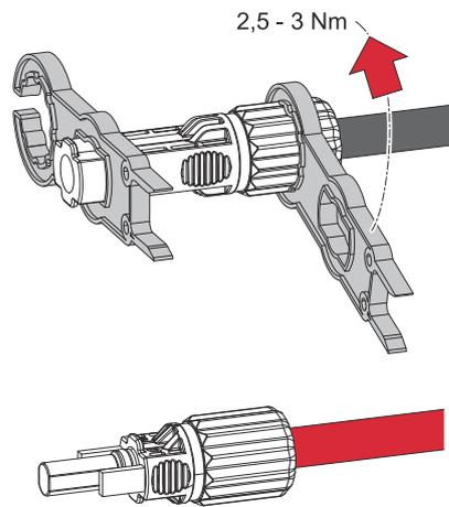
Tighten the cable gland using the supplied Amphenol plug tool to a torque of 2.5 Nm - 3 Nm.
