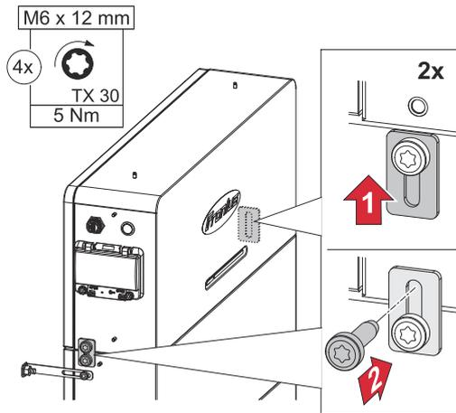
Fasten the 2 connecting tabs using the screws supplied (TX30) and to a torque of 5 Nm.
