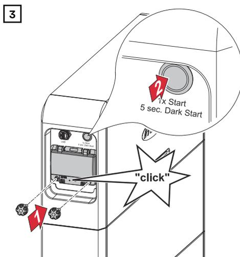
Close the cover of the DC disconnecter until there is an audible click and secure it against unauthorized opening with the screws. Press the start button once to start the battery.
