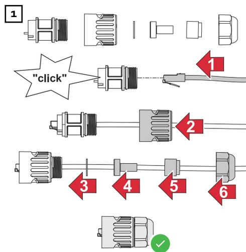
First, guide the data cable through the union nut, then through the seal and then through the cable gland. Fasten the union nut to the cable gland.
