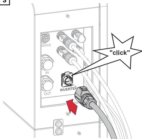
Connect the data cable to the "INVERTER" data communication connection until there is an audible click.
