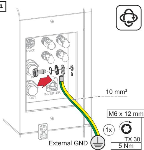
Fasten the ground conductor (PE) to the ground conductor connection using the screws supplied (TX30) and to a torque of 5 Nm.
