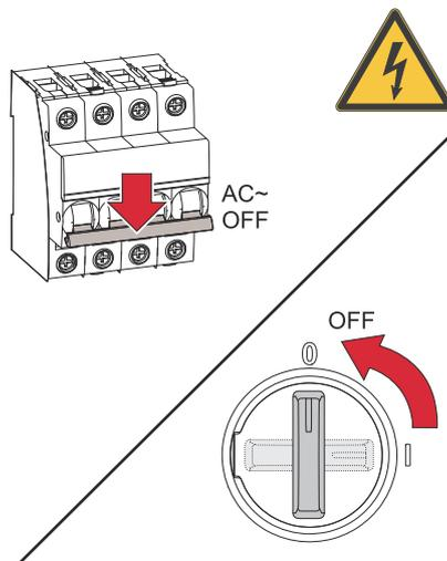
Turn off the automatic circuit breaker. Set the DC disconnect of the inverter to the "Off" switch position.
