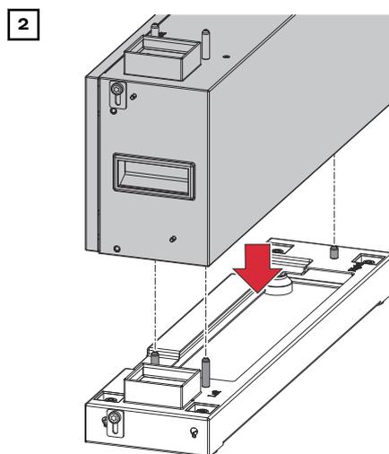
Place the Reserva module parallel to the base plate.
