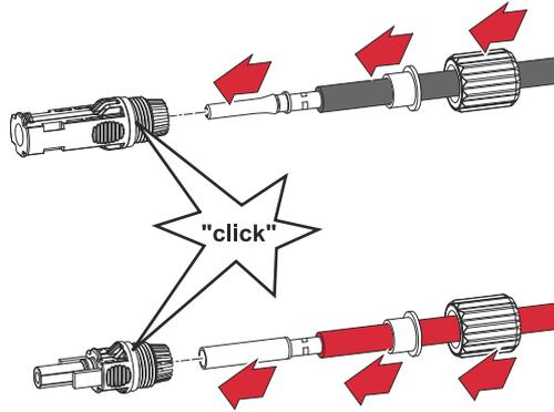
Guide the DC cable through the cable gland and the sealing ring. Crimp the crimp contact onto the stripped DC cable using a suitable Amphenol crimping tool. Push the crimp contact into the Amphenol plug until there is an audible click.
