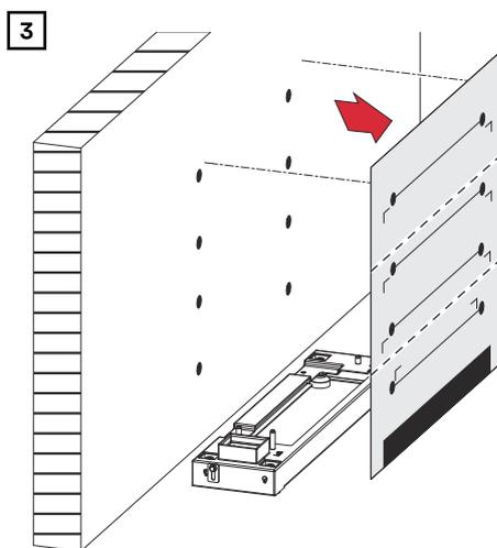
Carefully loosen the drilling template from the wall.
