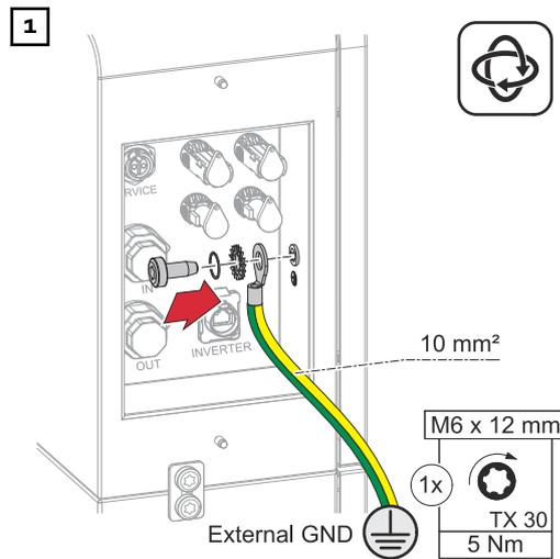
Fasten the ground conductor (PE) to the ground conductor connection using the screws supplied (TX30) and to a torque of 5 Nm.
