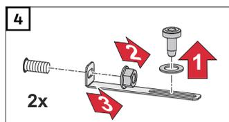
Loosen the L-shaped mounting brackets.
