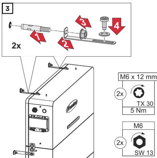
Fasten the L-shaped mounting brackets using the supplied screws (TX30), washers and to a torque of 5 Nm. Insert the bolt anchors into the wall and fasten with a socket wrench (width across flats 13).
