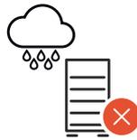
The battery is not suitable for unprotected outdoor installation.
