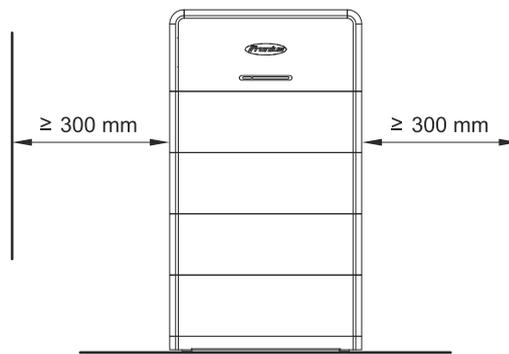
A minimum distance of 300 mm is recommended on the left and right side of the battery.
