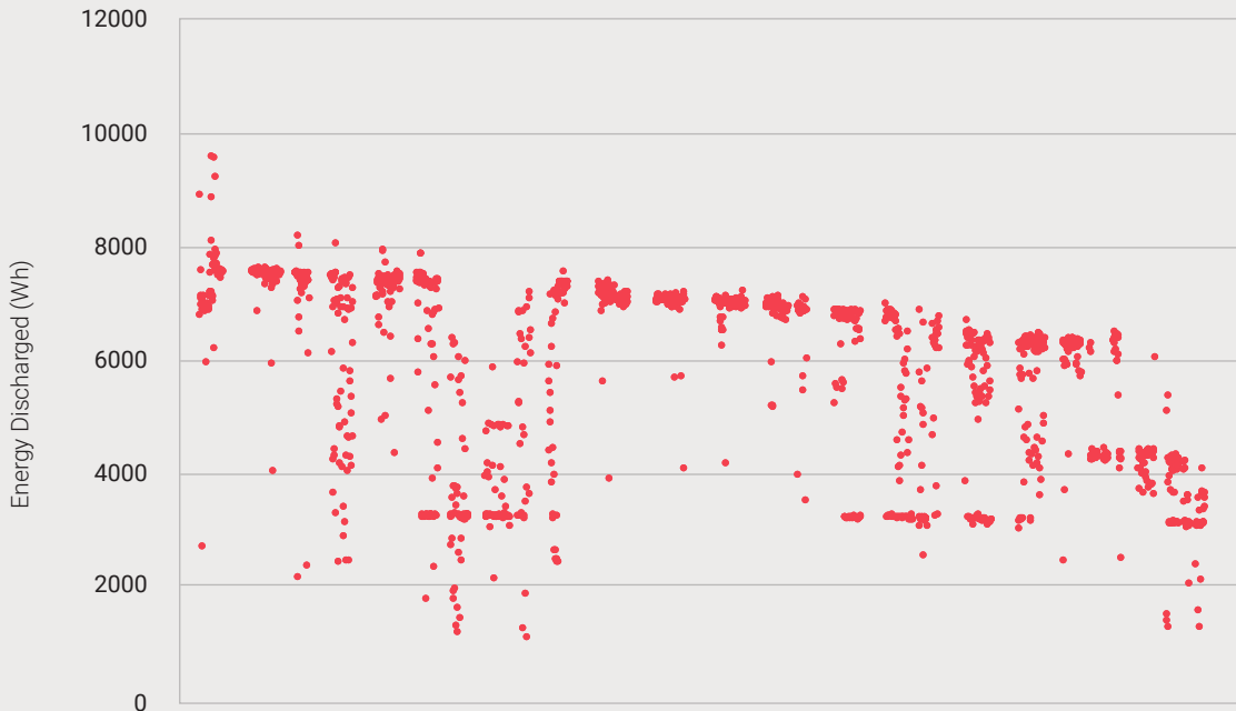
Figure 5. Energy discharged per cycle by the LG Chem RESU 1 battery pack
