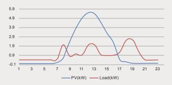
In the above scenario, families are much better off financially by installing a PV power generation system. But as shown in the figure, the consumption period of household loads does not match the output period of PV power generation well.
