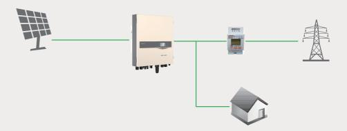
If the household loads and the PV generation curve are well matched, battery module may not be required, the SH5K hybrid inverter and meter could be used as a "Zero-export" system. In this system, the inverter output will be derated to ensure the feed-in power be zero when a feed-in power above zero is detected by the meter.
