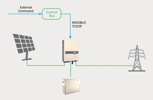
With the MODBUS TCP/IP protocol, the SH5K hybrid inverter can be manually configured via Control Box to shutdown, startup, active power derating, reactive power regulation, or charge/discharge power control etc..
