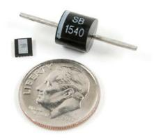
Figure 9. Solar cell optimizer IC from Maxim Integrated.
