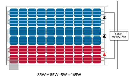
Figure 1. Performance of conventional module vs. solar cell optimizer module, when a single cell is shaded.
